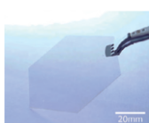
2-inch GaN crystal grown by the Na-flux method
